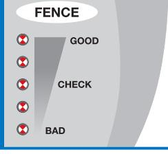
**If all are flashing, fence is operating correctly**
