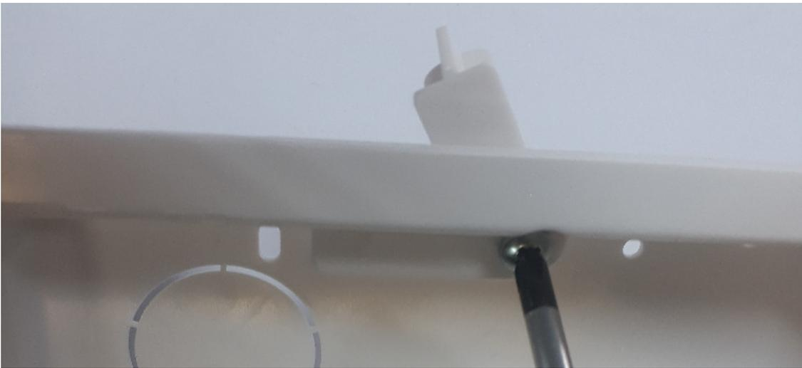
Wing clamp and Wing clamp screw
