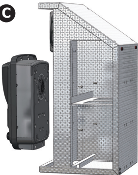
Energiser into the box (use 4 x M5x12mm Cap Screws)
